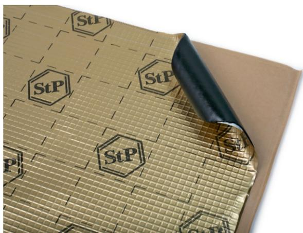
Multicomponent polymer based on butyl rubber supplemented with anticorrosive excipients. The material is a resinous construction of black color with the adhesive layer covered with corrugated aluminum foil of golden color with black printing and small cell stamping. The adhesive layer is covered with the antiadhesive paper to prevent contamination of material before its applying.
